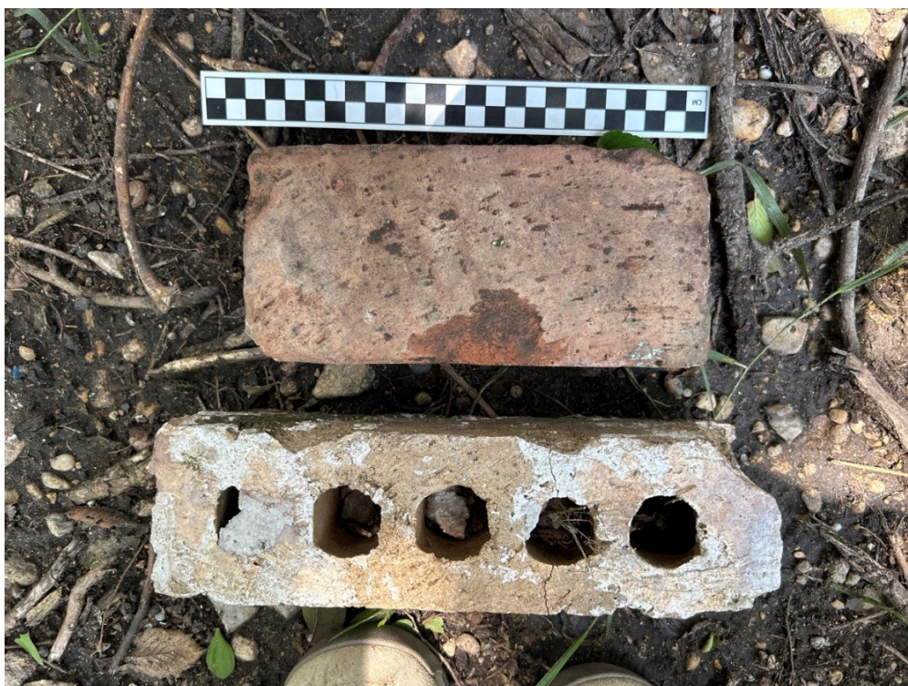
Figure 44: Machine-made red and extruded bricks (SF 02)
